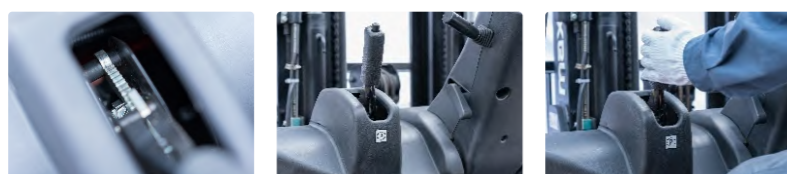
Hand brake use ratchet type (lighter and easier) ✓
