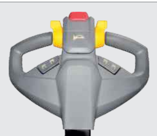
Centralized tiller for one-hand operation handle
